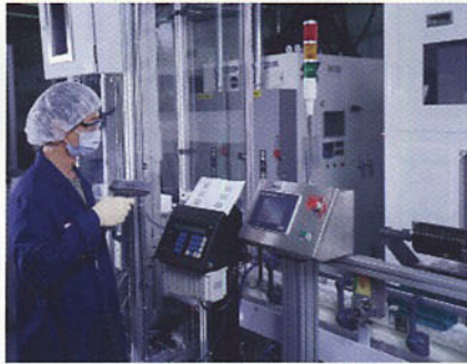
At the automated fab facility, data terminals function as a front-end data gathering mechanism for the MES. Although automated production doesn't require operators, they can use hand-held scanners and the data terminals to query the system about a given cassette, select processes to perform, and update lot status. (Photo courtesy Foto F/X, Les Baldwin)
