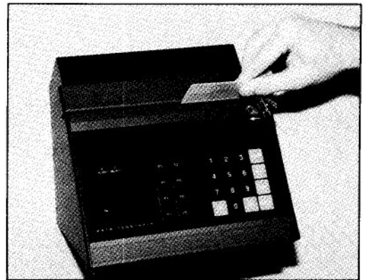
Data terminals read magnetic stripe badges to track time and labor for Nashua Photo.
